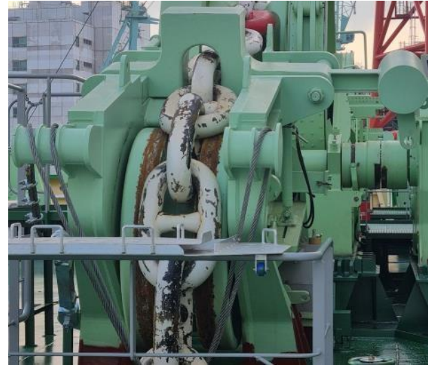
Anchor chain stopper for 147mm chain
