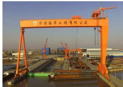
1000吨造船式龙门吊 1000t Shipbuilding Gantry Crane
