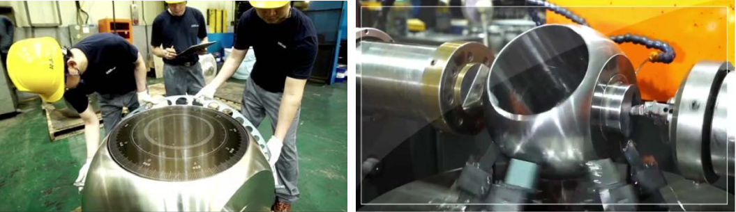
Superiority 2 : Super Fine Surface Finish Ra 0.05 μm
